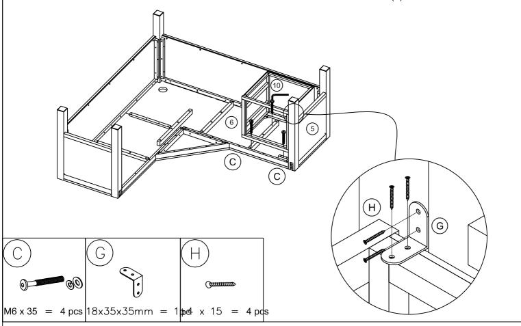
**STEP 8** FIXED THE DRAWERS BOX (10) INTO CASE SETUP.
